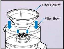
Place the Stainless Steel Filter Basket inside the Filter Bowl. With hands on outer edge, press Filter Basket down firmly to latch into position.
